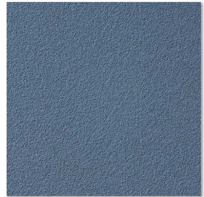
Juraku Type of aggregates: Marble powder No.1
