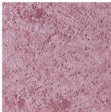
Press-L Type of aggregates: Marble powder No.5, No.8
